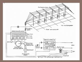
SAQ Grimeton operates at 17.2 kHz (VLF) with a 200 kW Alexanderson alternator and a 2.2 km long antenna, using Morse Code. Built in 1922-1924, it is now on the Unesco World Heritage List.
